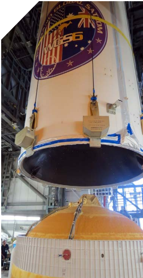
The Department of Defence Wideband Global Satellite 6 (WGS6) satellite as its being connected to the launch vehicle in preparation for take-off. Image courtesy of Boeing. (Department of Defence)
