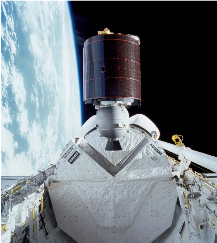
Australia's AUSSAT communications satellite is deployed from the payload bay of the space shuttle Discovery (NASA)
